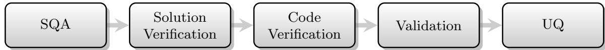
Figure 3.1: General process for establishing code credibility. Each of the five steps minimizes different sources of uncertainty and is described at length in this chapter.
